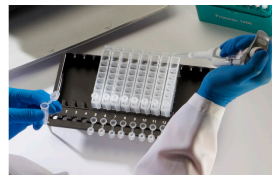
Prepare your sample, add it to a cartridge and load it into the Maxwell® RSC.
