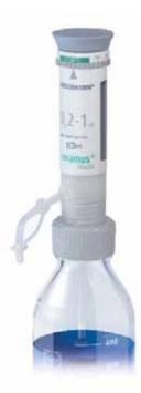
With ceramic pistons. High precision, bottle-top dispenser, adjustable in fixed steps for the reproducible dispensing of liquids. Declaration of conformity acc. to DIN 12600. With patented, high-purity, alumino-ceramic pistons and highly polished, DURAN® glass cylinders, guaranteeing continual durability and precision.
