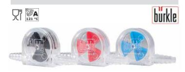
Gives a visual indication of liquid or gas flow in tubing. Operates in both directions and at any angle. Can accomodate flow rates down to approx. 150 ml/min. Length incl. nozzle 88mm. For tubing from 6 mm to 11 mm diameter. Maximum pressure: 2 bar. Food Safe.
