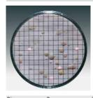
Sterile, dehydrated culture media pads in petri dishes. Once they are moistened with 3.0 ml to 3.5 ml of sterile and demineralised (or distilled) water they are ready-to-use immediately. All Nutrient Pad sets are supplied with the appropriate membrane filters, which are also individually sterile packed. Shelf life of the NPS 18 to 24 months at room temperature.
