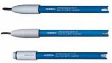
Basic pH combination electrodes, with plastic body and gel reference system. SenTix® 20 with plug head (AS/DIN (9.040 895) or AS/BNC (9.040 897) cable combination please order separately). Sentix 21-3 and Sentix 41-3 with 3 m fixed cable.
