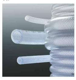
Transparent. Supplied per 10 metre. PVC with terylene mesh reinforcement. Certificated by German TÜV with due regard to regulatory of DIN EN ISO 5774:2008. Proofed by BGVO directive 2002/72/EC bis 2008/39/EC for food contact. Durometer 77 Shore A.
